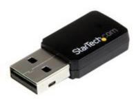
The USB433WACDB USB 2.0 Mini AC600 Wireless Network Adapter lets you add Wireless-AC connectivity to a desktop or laptop computer, through a conveniently small USB adapter.
