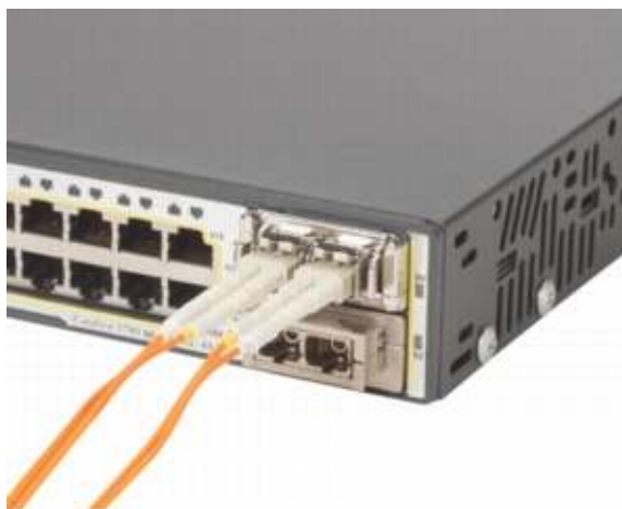
Figure 4. Cisco TwinGig Converter Module converts each 10 Gigabit Ethernet X2 Interface into Two Gigabit Ethernet SFP Ports with Catalyst 4500 Supervisor 6-E
