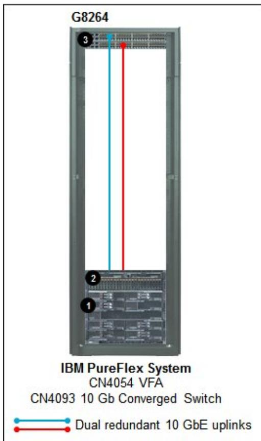
Figure 6. CN4093 Virtual Fabric in the Full Fabric mode (end-to-end FCoE)
