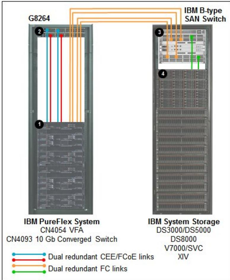
Figure 7. CN4093 as an NPV Gateway connected to the IBM B-type SAN
