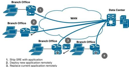
Figure 2. Using the Same Cisco SRE Infrastructure for Different Applications
