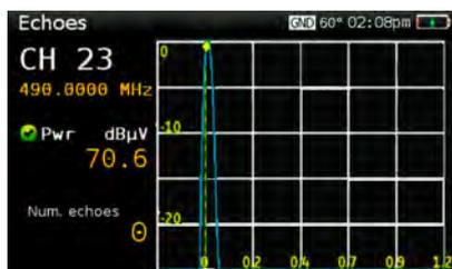
In terms of terrestrial signal reception, controlling the absence of any echoes that could jeopardize reception is crucial. H30Crystal displays the echoes of the received signal, allowing the installer to minimize them for optimal signal reception.
