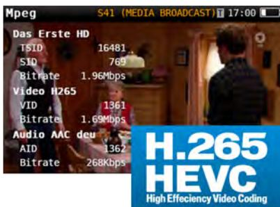
This functionality supports HEVC H.265 new compression format and allows to display video signals with a maximum Full HD resolution (1920 x 1080). Information can be displayed both on the meter screen\* or on the mobile device (multiscreen mode) as long as your hardware is H.265 compatible (usually a smartphone, tablet or PC).
