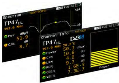
This functionality for DVB-S/S2 allows the complete analysis of a satellite channel in any frequency within the 250 MHz to 2300 MHz range. Thus, the meter can be directly connected to any output of a LNB Wideband (2 outputs: Vertical and Horizontal)
