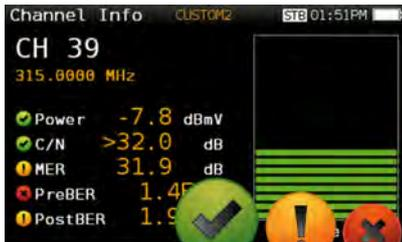
Reduce installation mistakes with the on-screen Pass/Fail indicators, a graphical tool that helps and speeds up the interpretation of measurement results. Different thresholds are available depending on the network area to be analysed: headend, multi-band amplifiers, bridging connection, connection records, user home, etc. Besides the pre-set values, you will be able to customize your own threshold values.
