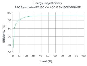
Curve fit to measured efficiency data. All measurements taken in normal operating mode, at typical environmental conditions, with nominal electrical input and balanced resistive load (PF = 1.0) output
