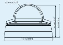
AXIS P3346/-V AXIS P3346 weight: 490 q (1.1 lb.) AXIS P3346-V weight: 700 g (1.6 lb.)
