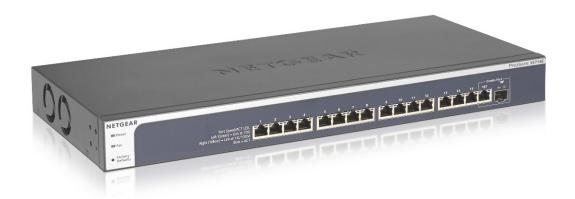
The ProSAFE® XS716E 10-Gigabit Ethernet Web Managed Switch, like the XS708Ev2, uses 2<sup>nd</sup> Generation 10-Gigabit Ethernet technology. The XS716E has 16 copper 10GBASE-T ports with one shared (combo) port supporting 1G or 10-Gigabit SFP+ fiber modules (either Port 16T or Port 16F may be used as a copper or fiber connection to network).
