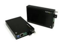
The ET90110WDM2 10/100 Mbps Ethernet Single Mode WDM Fiber Media Converter Kit SC (20km) lets you extend a 10/100 Mbps Ethernet connection over single mode fiber, at distances up to 20 km (12.4 mi).
